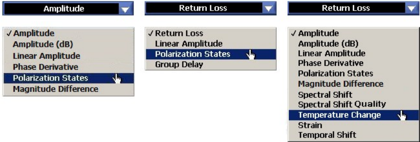
Figure 3-6. The parameters menu on the left is available for the upper graph. The menu on the right is the Time Domain menu for the lower graph area. The last five parameters will be gray (unavailable) in some models. By selecting Frequency Domain in the top right corner of the lower graph area, the menu shown in the center becomes available.
