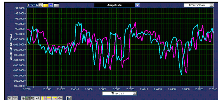
Figure 4-12. The reflection Amplitude for the same temporal range as in Figure 4-11 for Trace A (blue) is shifted by roughly -0.8 fs to the left of the Shift Reference, Trace E (purple).
