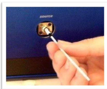
Figure 6-6 Cleaning Optical Bulkhead Connections using a Cletop Stick
