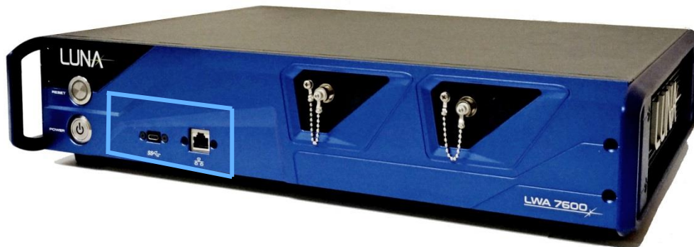
Figure 3-2 – LWA 7600 USB and Ethernet Connections, shown in blue box.
