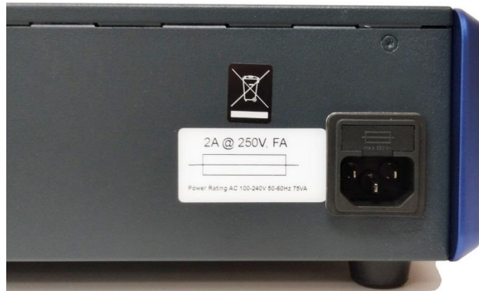
Figure 3-4 LWA 7600 Rear Panel Power Entry.
