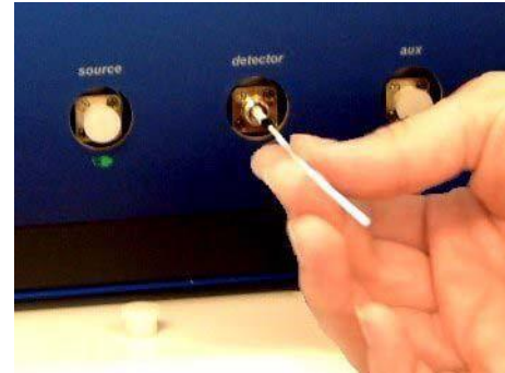
Figure 10-1. Remove plastic cap from the bulkhead connectors. Gently insert supplied mini foam swab, rotate in one direction, then remove. Use a new swab for the next connector.
