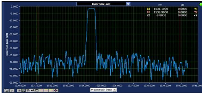
Figure 5-8. Graph window with vertical cursors appearing at the default location. The legend at the upper right gives the precise location of the cursors and the distance between them (dX in this case).
