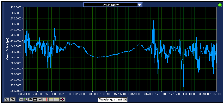
Figure 5-16. Group delay data for a Bragg grating reflection (sample data file “Bragg Reflection.dat”) before filtering.
