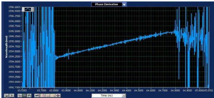
Figure 7-23. Phase derivative of the time domain response of a fiber Bragg grating.
