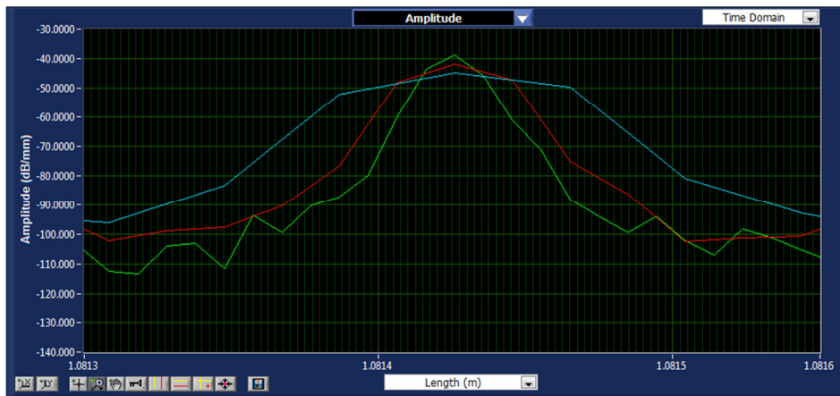
Figure 3. Close-up of the jumper connector reflection shown in Figure 1, Amplitude (dB/mm) scaling, taken with a wavelength range of 21 nm (blue), 43 nm (red), and 88 nm (green).
