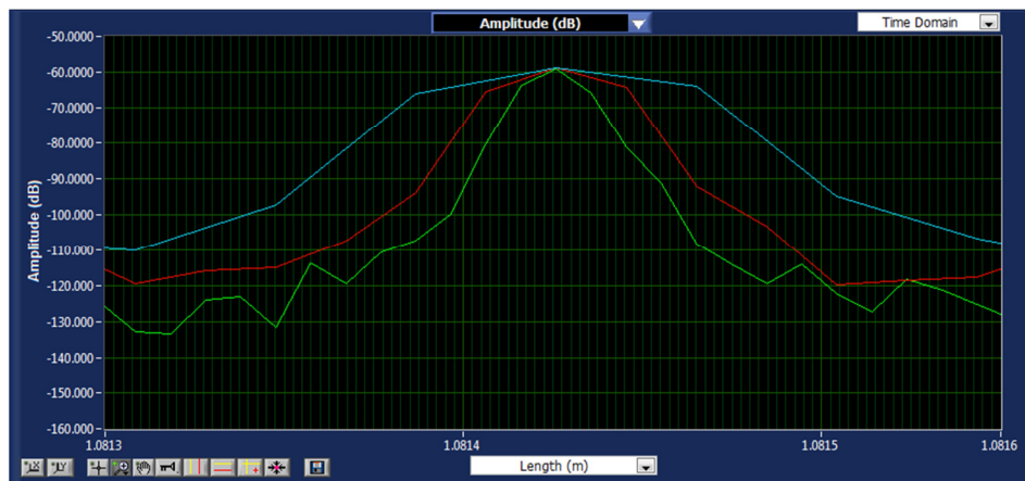
Figure 4. Close-up of the jumper connector reflection shown in Figure 2, Amplitude (dB) scaling, taken with a wavelength range of 21 nm (blue), 43 nm (red), and 88 nm (green).
